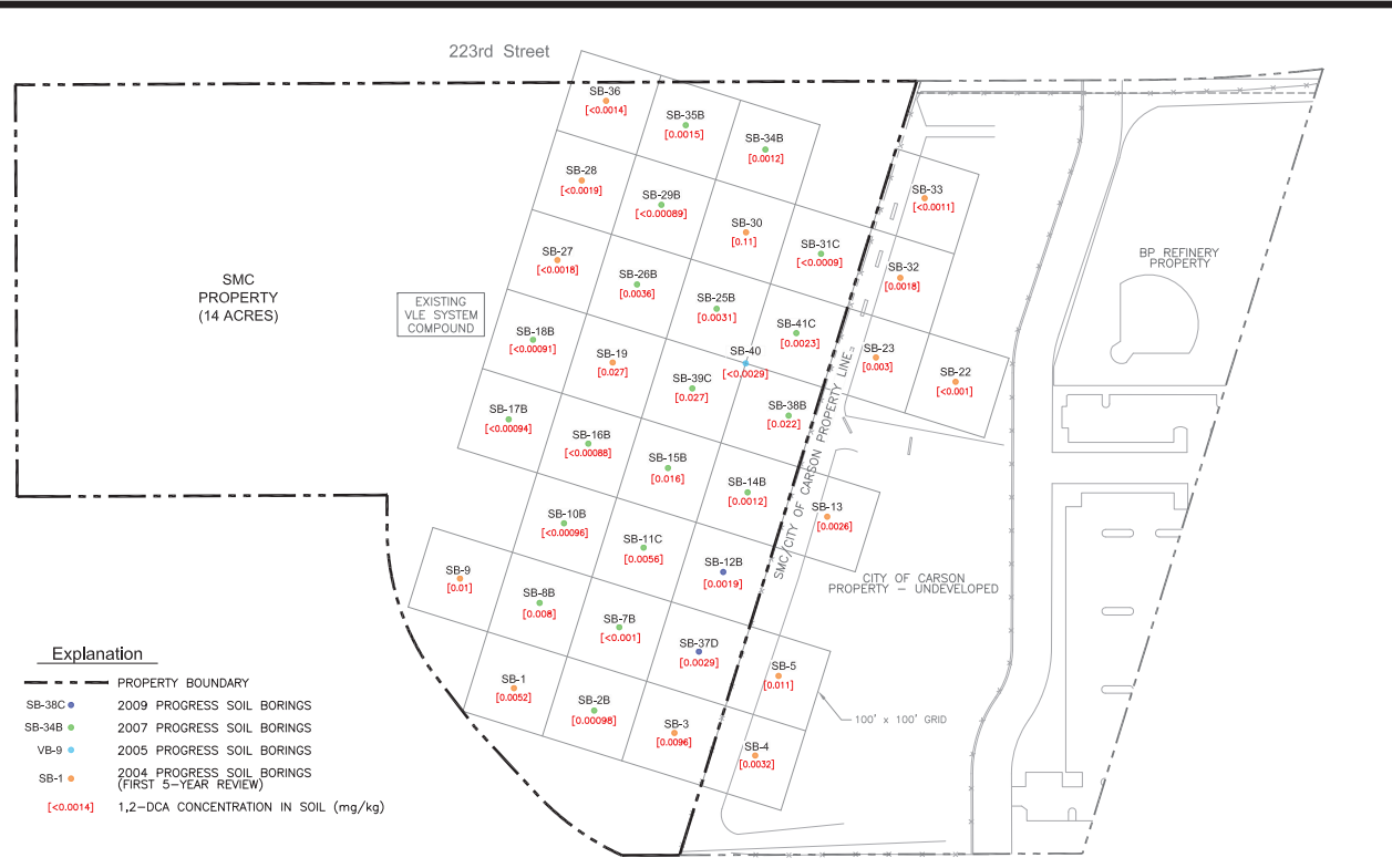
1,2-DCA IN SOIL 0-15 FEET BGS
