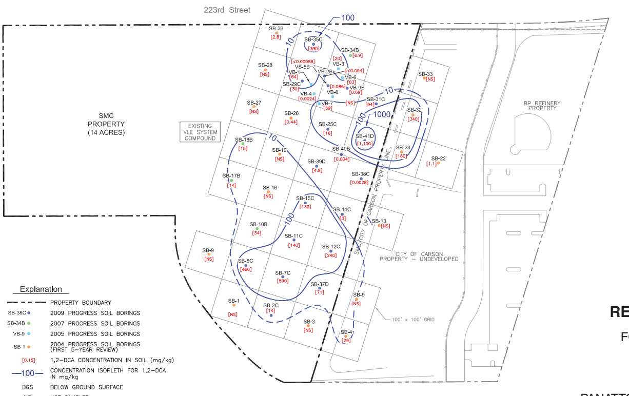
1,2-DCA IN SOIL 35 FEET BGS
